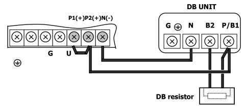
3.3.7 Wiring guide when using both of DC reactor (Option) and DB Unit(option) (AC power input: 30kW and higher)
