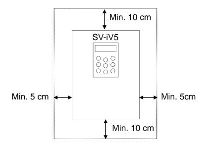
At least the room that 30 cm from upper and lower of inverter and 20 cm from left and right of inverter is required for installing more than 30 kW products.
