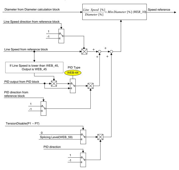
Line Speed Command Block Diagram
