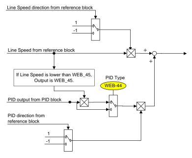
PID Type Block Diagram
