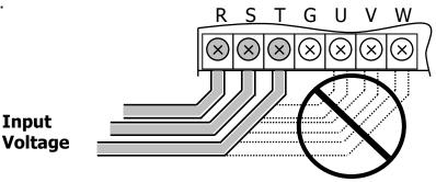
② Never connect the phase advancing capacitor to the inverter output. If already installed, remove the phase advancing capacitor clearly.
