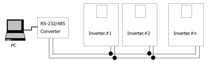
RS-485 terminal connection: connect to S+, S- of the terminal block (see Chapter 4 Wiring)
