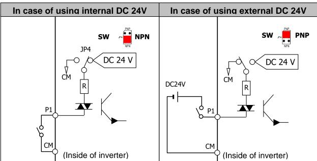
Guaranteed PNP type input voltage (external DC 24V): On voltage (DC 19~25.2 V)/ Off voltage (DC 7V or less)
