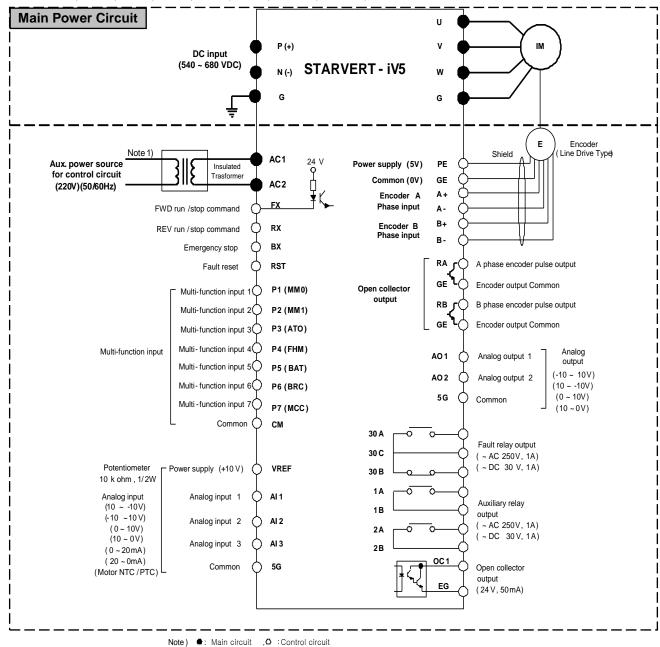
Note 1) It is used when inverter control circuit is energized from auxiliary power source (220 VAC) without main power supply. Use insulated transformer to separate from main power supply. (Transformer capacity: above 100VA recommended)
