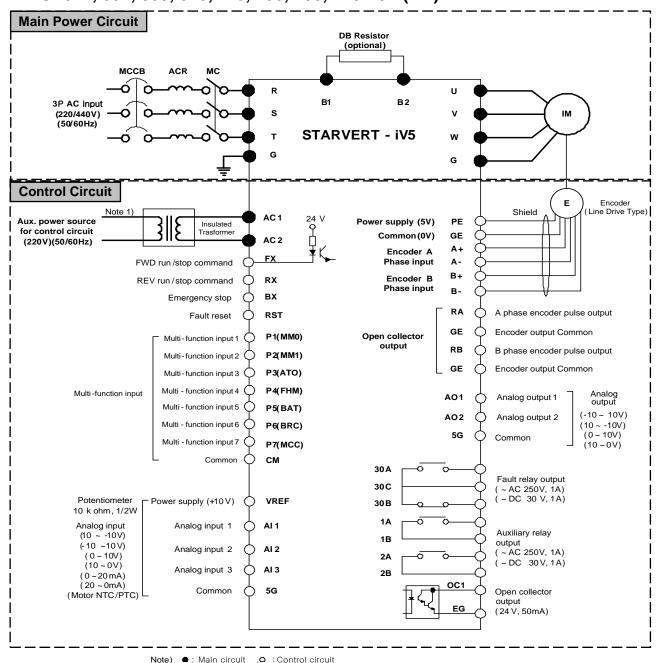
Note 1) It is used when inverter control circuit is energized from auxiliary power source (220 VAC) separated from main power supply. Use insulated transformer to separate from main power supply. (Transformer capacity: Above 100VA recommended) Only 11~22kW-2(Press) and 5.5~22kW-4(Press/Mold) supported (Other products will be released later.)
