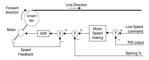
Figure 3. Roll Rotating Direction at the time of Unwind/Overwind Setting, Forward Direction Operation Command
