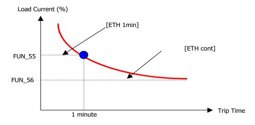
[Motor i2t Characteristic Curve]
