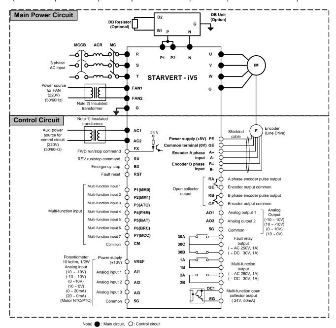
Note 1) It is used when inverter control circuit is energized from auxiliary power source (220 VAC) without main power supply. Use insulated transformer to separate from main power supply. (Transformer capacity: above 100VA recommended)
