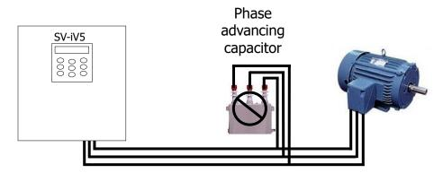
③ Cable between inverter output and motor should be less than 30m long. If cable gets long, surge voltage appears across motor terminals depending on the cable parameters. Especially, in 400V class motor case, insulation withstanding voltage may be decreased. Use an insulation-enforced motor when 400V class motor is used.
