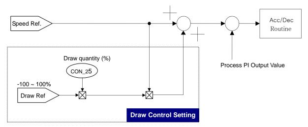
One of the multi-function analog input is set to the draw command ranging from -100% to 100% and the speed command multiplied by Draw quantity is added up to the speed command (Speed Ref) to obtain the final speed command. That is,  $-100 \sim 100\%$  of the Draw command value is scaled to the Draw quantity (%) of CON\_25, which is multiplied with the speed command value to produce the command value which is proportional to the speed command value.
